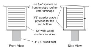
Figure 5.2; Standard enclosure for temperature sensor
