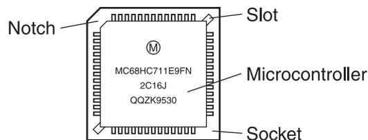
Figure 3; Microprocessor installed in PLCC socket
